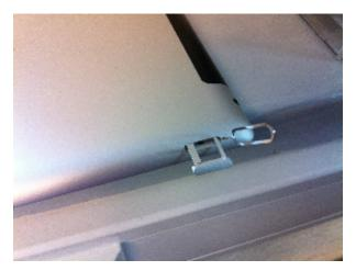
Set the micro-SIM card in the bay as shown in the picture (it fits in the holder only in one position) and push the holder back in the device:
