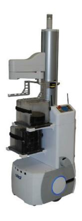
The Omron Adept Lynx™ Semi Handler combines a Lynx autonomous indoor vehicle (AIV) with a collaborative 4-axis robot to produce a highly versatile mobile robot designed to pick, place and move semiconductor waferpods throughout a wafer fab. It is designed to exchange wafer pods from a variety of processing equipment, stockers and storage (WIP) racks, and operates collaboratively within a fleet of Lynx vehicles.
