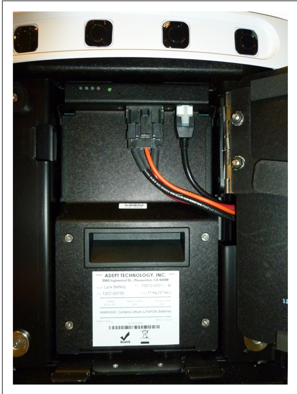
Figure 2-4. Battery Compartment, Connectors
