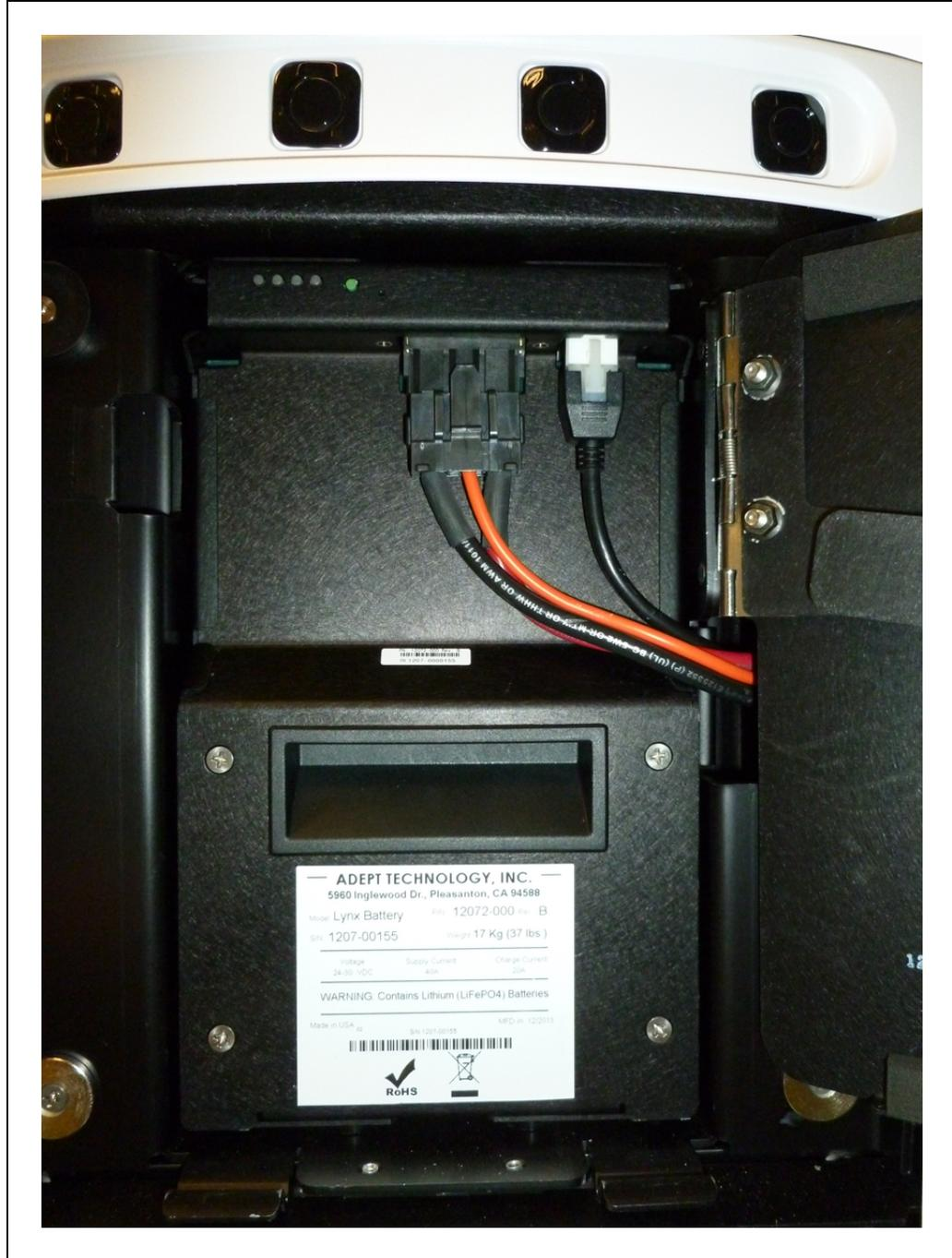
Figure 8-6. Battery Compartment, Connectors
