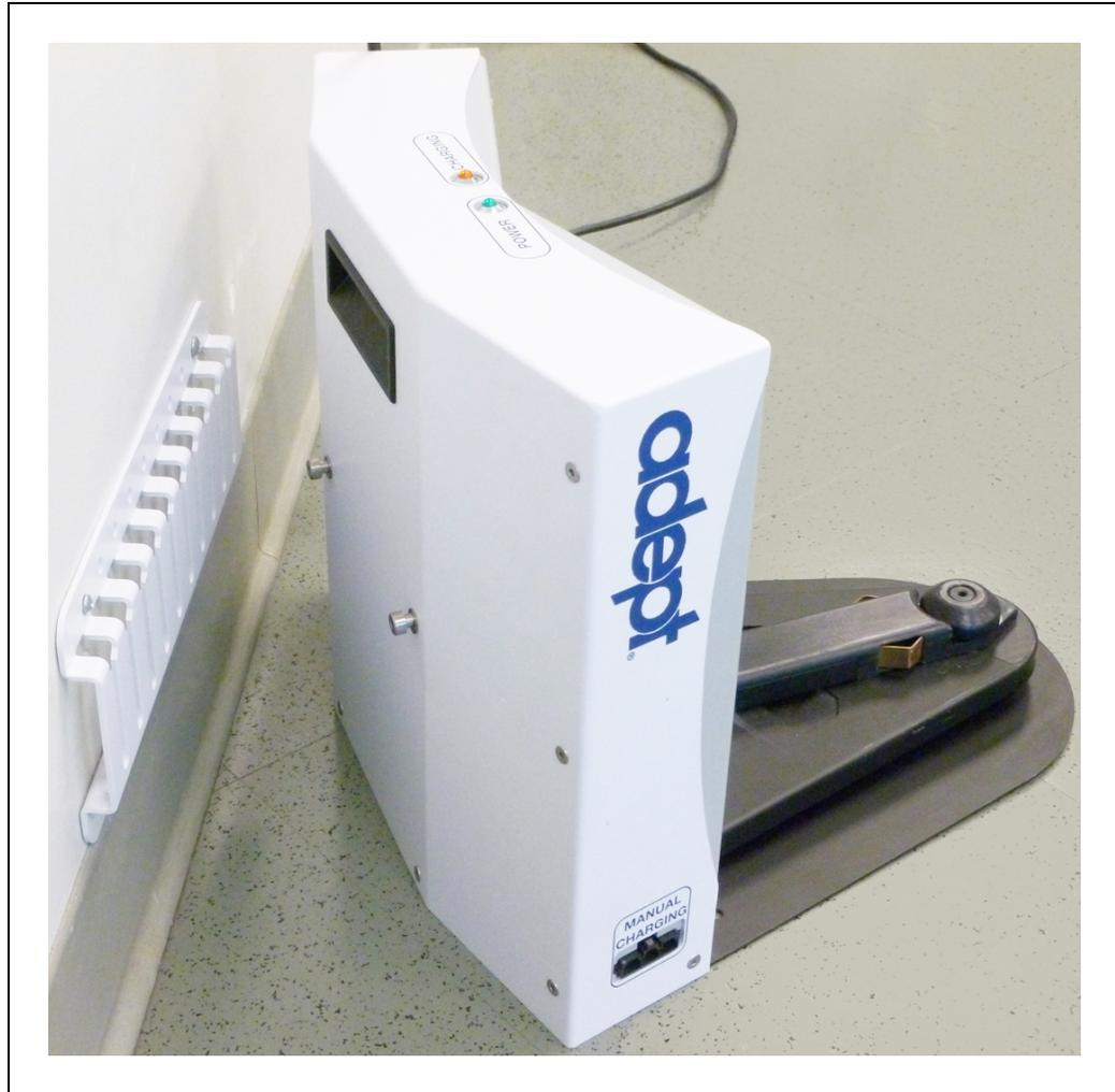
Figure 2-9. Rear View of Docking Station with Wall Bracket
