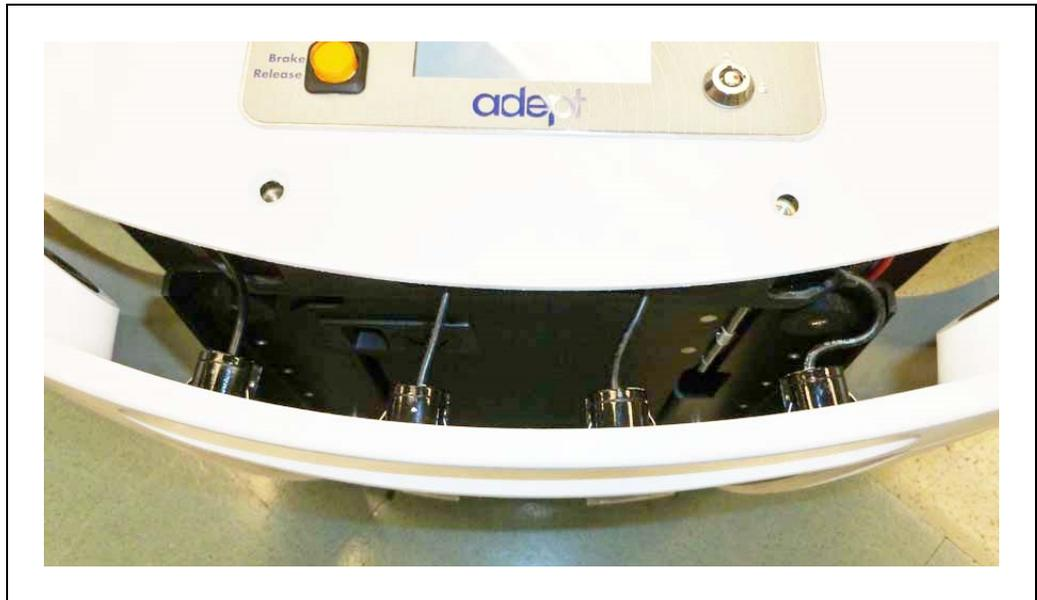
Figure 8-2. Sonar Leads, with Connectors Still in Chassis
