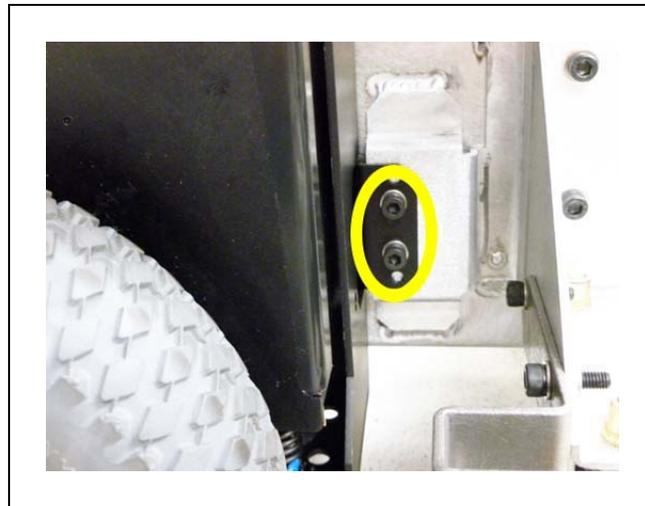
Figure 8-16. Mounting Screws at Bottom-Right of Drive Assembly
