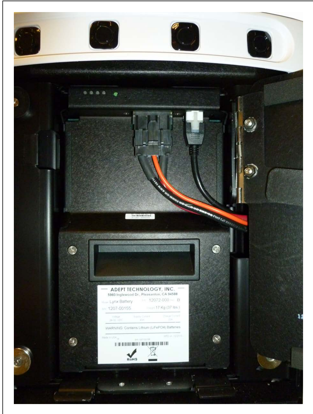
Figure 3-8. Battery Compartment, Connectors
