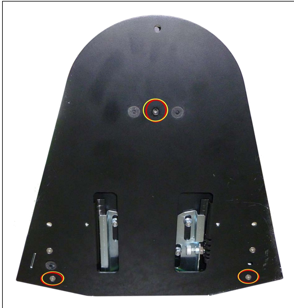
Figure 3-15. Underside of Docking Station Foot, Showing Screw Locations
