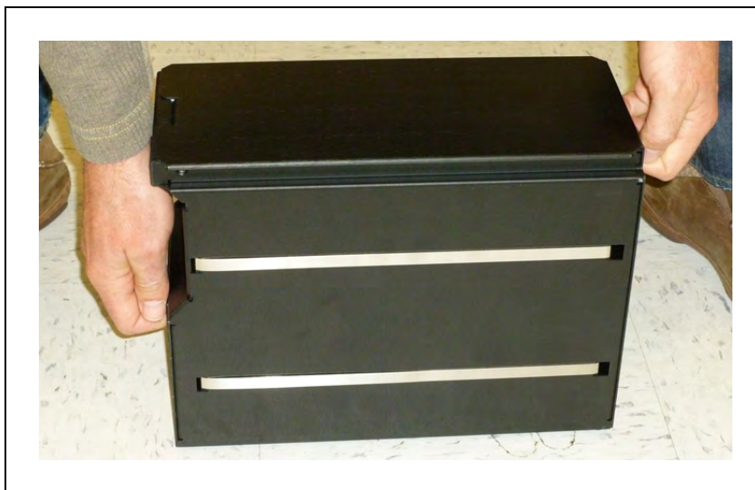
Figure 2-7. Lifting the Battery
