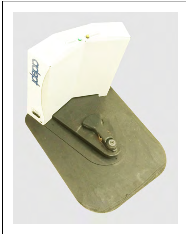
Figure 2-12. Docking Station, Mounted on Floor Plate
