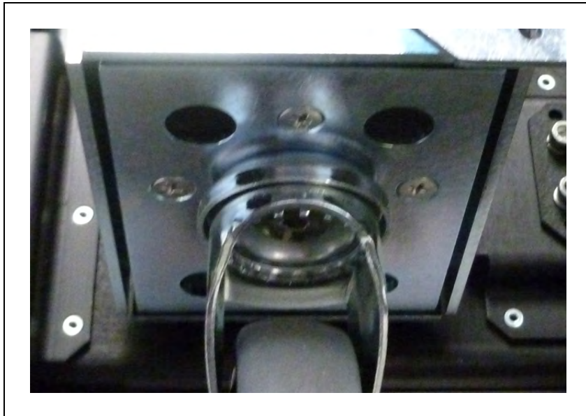
Figure 8-15. Rear Caster Attachment
