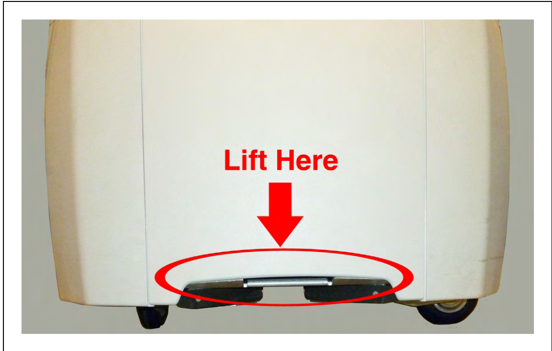
Figure 2-4. Bottom of Inner Rear Cover. Lift from the Frame, not the Cover.
